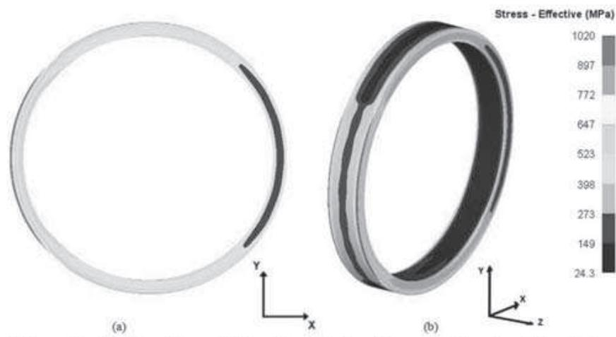
Figure 11 – Residual stress in the distorted ring after quenching simulation: (a) top and (b) 3D views.
