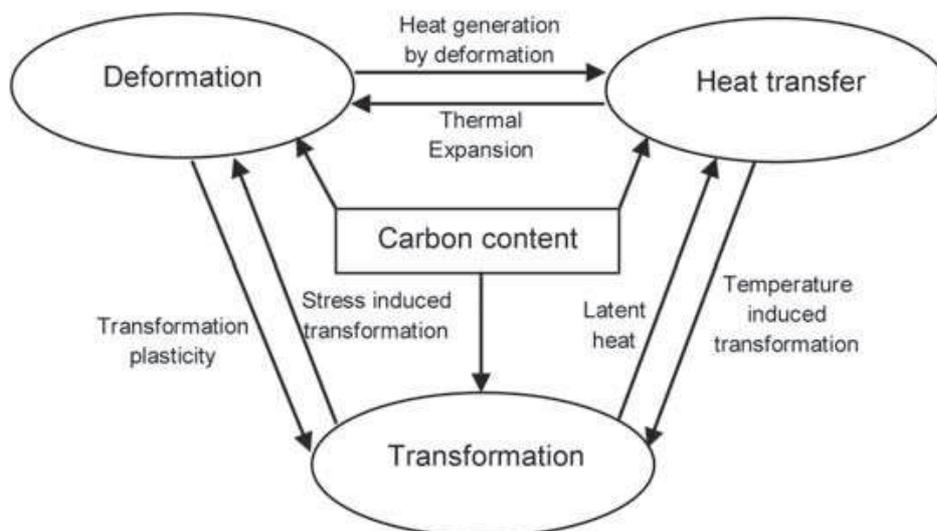
Figure 1 – Coupled phenomena considered during the quenching simulations.
