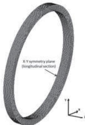
Figure 6 – Meshed 1/2 ring symmetric geometry used for the simulation.
