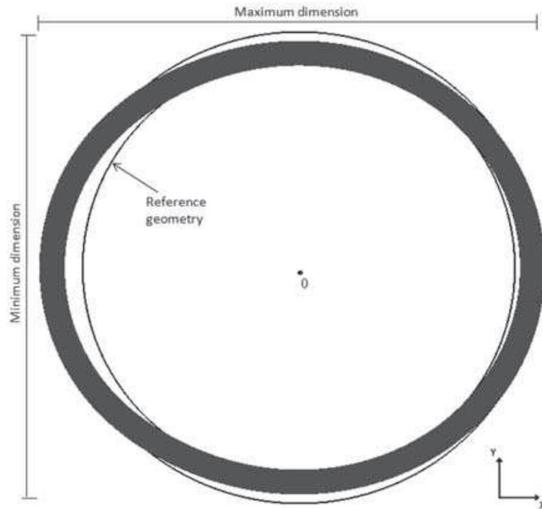
Figure 10 – Quenched distorted ring for hypothetical case (displacement magnified 10x).
