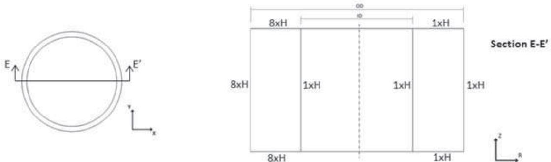
Figure 9 – Schematic drawing of the ring's cross section showing the heat transfer coefficient distribution on the surface.
