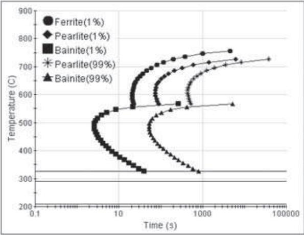
Figure 2 - TTT diagram of 4140 steel calculated by JMatPro.
