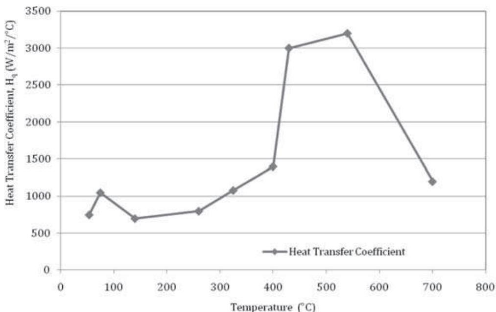
Figure 7 – Heat transfer coefficient for quenching solution from supplier company [12].
