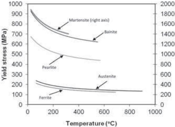
Figure 3 - Proof stress of various phases during cooling at 10°C/s.
