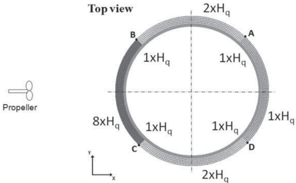
Figure 8 – Heat transfer coefficient distribution on the ring surface. Inside surface is represented by a green line; and regions DA (green), AB and CD (yellow), and BC (red) represent the surface regions referred to top, bottom and outside surfaces.
