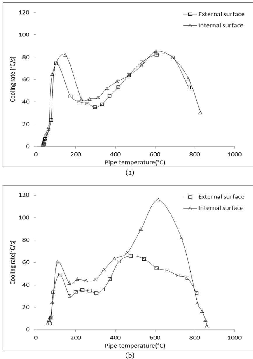
Figure 4 – Cooling rate during the quenching process at: (a) leading end and (b) tailing end.
