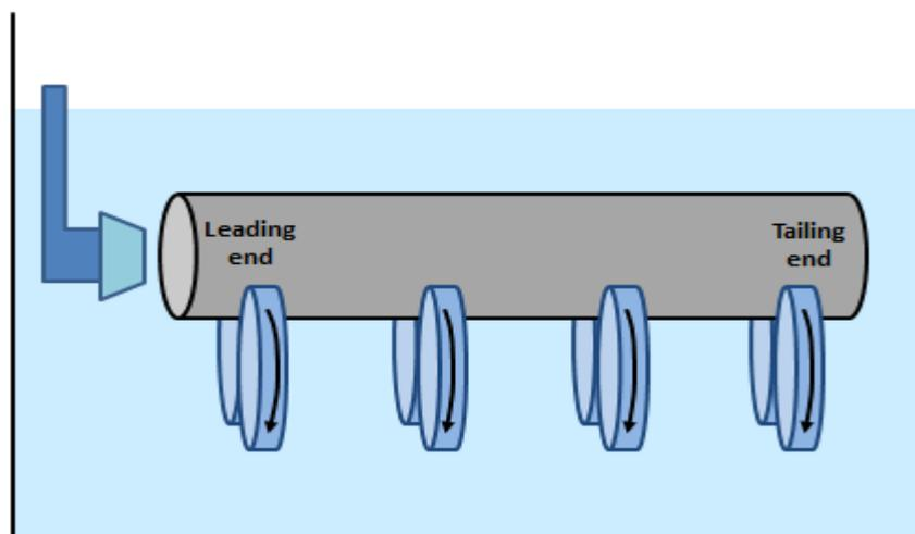
Figure 3 – Pipe positions for measuring the cooling curves into the quench tank.
