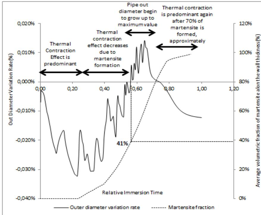
Figure 7 – Outside diameter variation and volumetric fraction of martensite distribution along the wall thickness.
