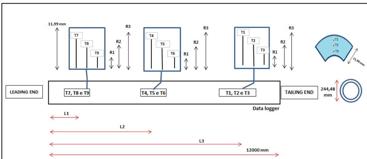
Figure 1 - Schematic pipe assembly used in experimental test
