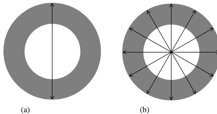
Figure 2 – Out diameter equipment's (a) Example of Zumbach measurements (b) Example of IMS OD Machine measurements
