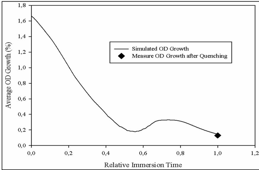
Figure 5 – Simulated outside diameter growth behavior at the leading end during quenching process.
