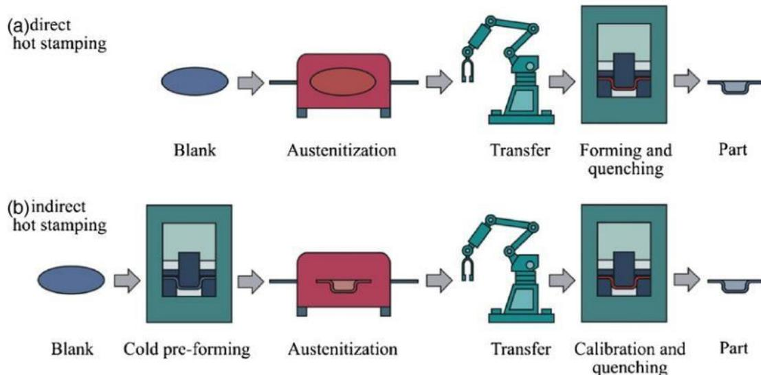
Figura 1 – Basic hot stamping process chains: (a) direct hot stamping (b) indirect hot stamping (adaptado do artigo “A review on hot stamping”, Journal of Materials Processing Technology, H.Karbasian, A.E.Tekkaya, 2010)
