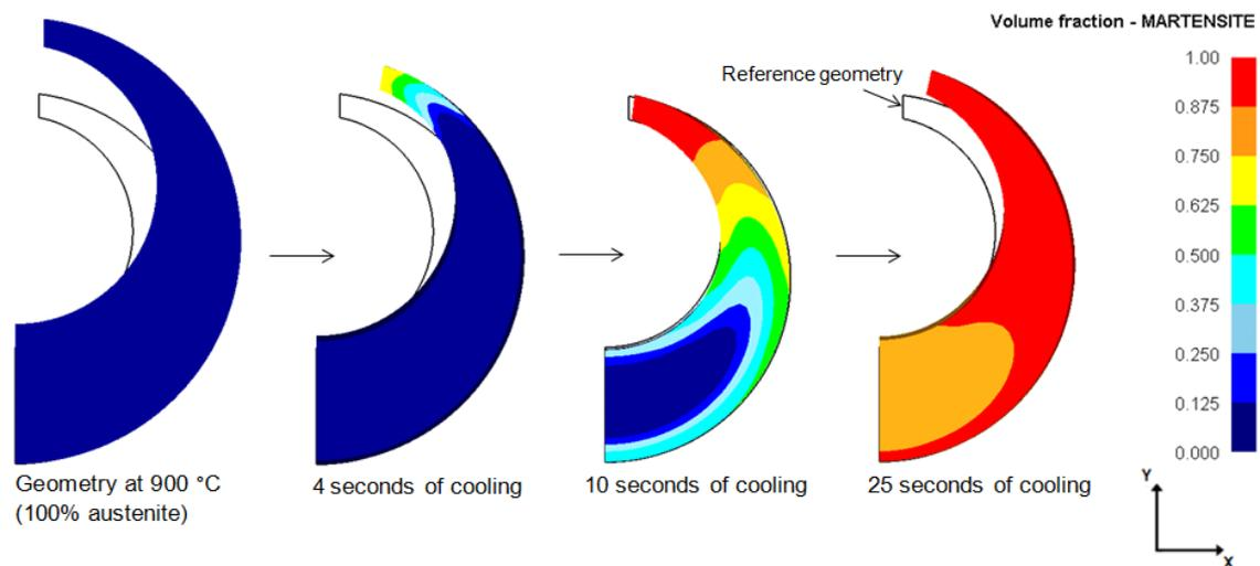
**Figure 12.** Martensite formation on the C-ring during the cooling simulation for oil quenching (displacement magnified 20x).
