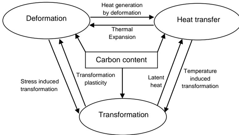
**Figure 3.** Coupled phenomena considered during the quenching simulations.
