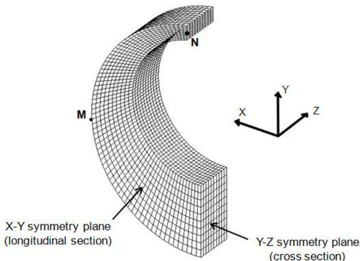
**Figure 7.** Meshed  $\frac{1}{4}$  symmetric geometry, used for the simulation. Nodes *M* and *N* were used for outside diameter and gap opening evaluation, respectively.
